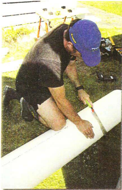
Saw 30mm VC cylinder to size.
